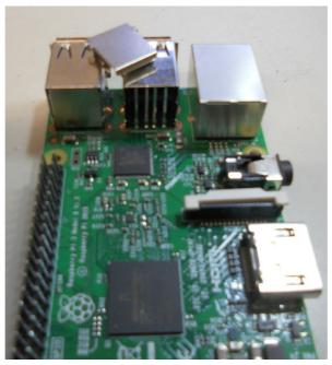
Remove the shield cover from the back of the USB port
