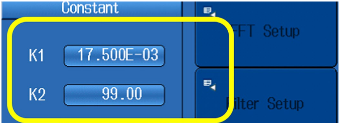
Figure 21. Constants for equations K1 (degrees to radians conversion) and K2 (sensor angular offset in degrees).
