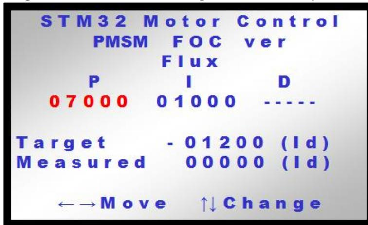
Moreover, to achieve speed regulation in speed control mode, a PI is also implemented. The tuning of its related gains can be done in real time by means of the dedicated LCD menu:
