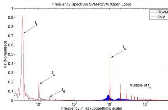
Figure II-34: SVM, RSVM; Frequency Spectrum Contrast
