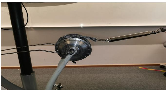
Figure 7: Experimental setup to determine the relationship between current and force.
