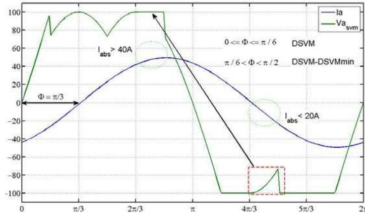
Figure II-5: Intelligent Switching Function -  $\phi > 30^\circ$
