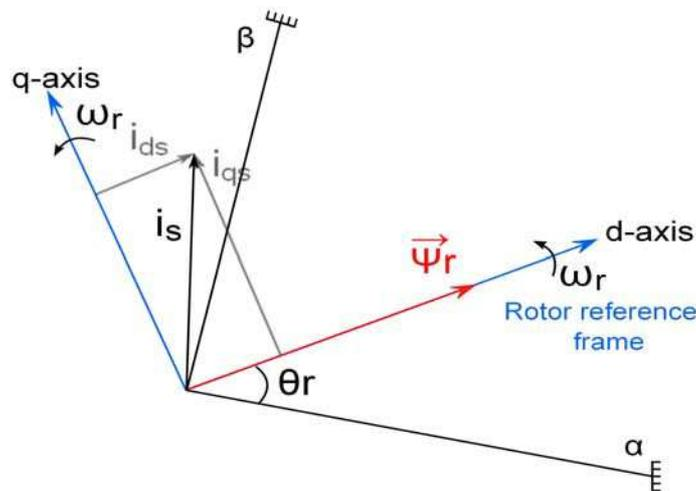
Figure II-16: FOC Phasor diagram
