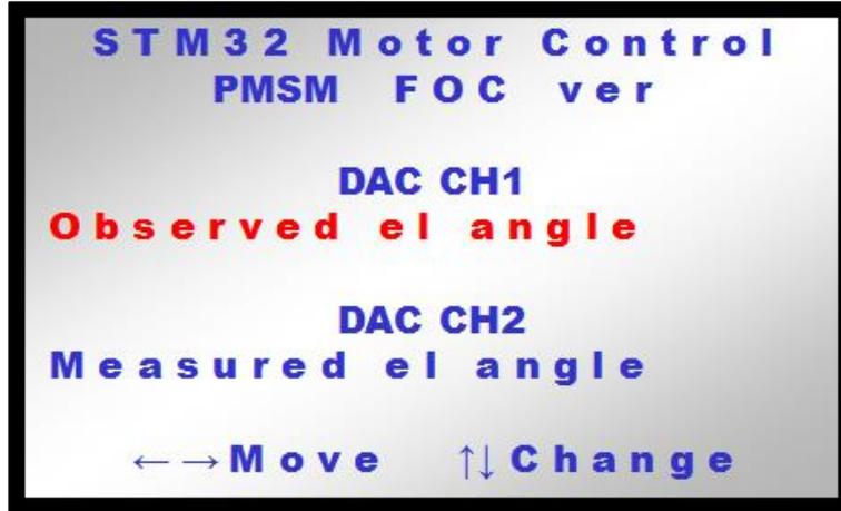
When the menu in [Figure 125: "LCD screen for setting the P term of the flux PID"](#) is displayed, the joystick can be moved to the right/left to select the desired DAC channel. To change the software variable in output, move the joystick up/down (the list of the available variables depends on the selected firmware configuration). For all other menus, pressing the joystick or the Key button will cause the motor to start/stop.
