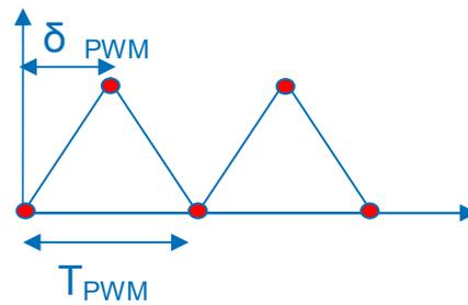
Figure I-24:Carrier signal randomization
