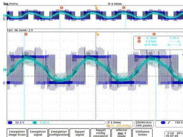
Figure III-53: Vector controlled EDSVM: Phase voltage and current
