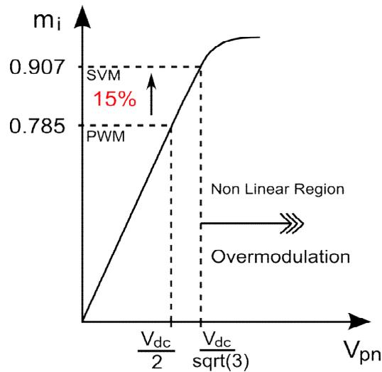
**Figure I-22: Increased linearity of Modulation Index**
