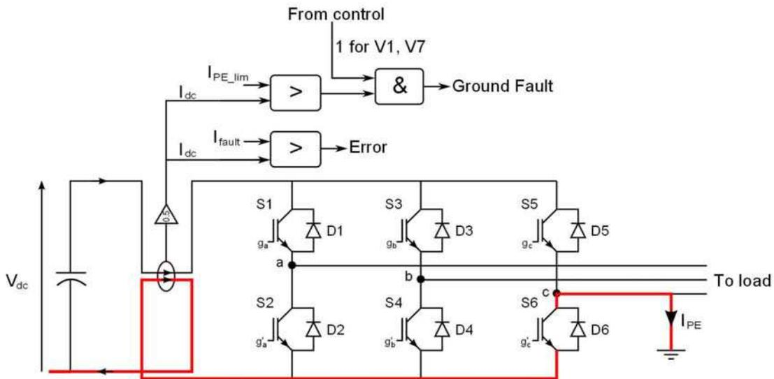
**Figure II-49: Ground Fault**
