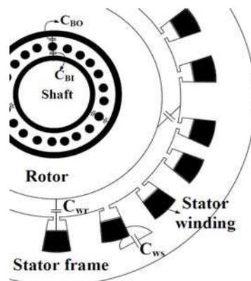
Figure I-33: High frequency model of an electric motor
