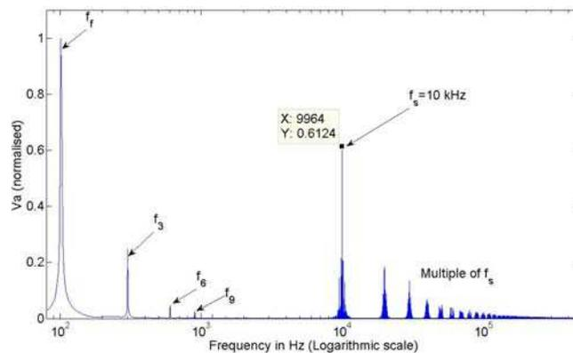
Figure I-21: Frequency Spectrum - Phase Voltage  $V_{a0}$
