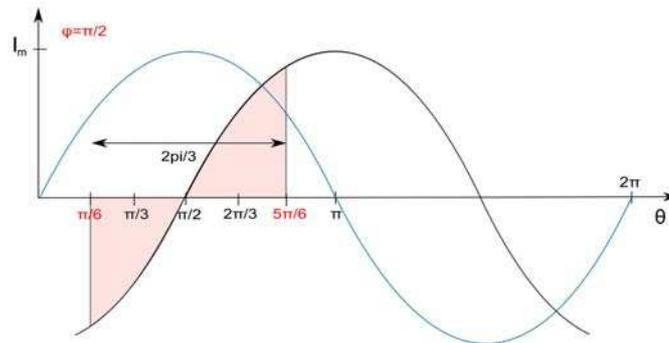
Figure II-9: Switching loss reduction  $\varphi=90^\circ$
