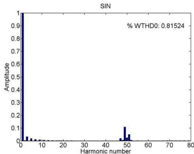
Figure III-23: SPWM: Harmonic spectrum
