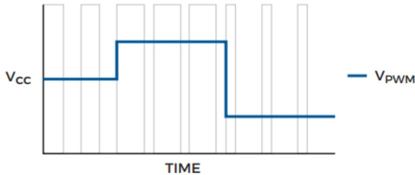
**Figure 7. Relationship between wave duty cycle and PWM output voltage**
