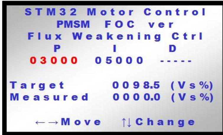
The target and measured stator voltages are shown in the lower part of the screen as a percentage of the maximum available phase voltage.
