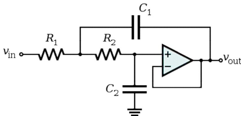
Figure III-13: Anti-aliasing filter
