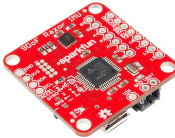
**Figure 4.6.** SparkFun 9DoF Razor IMU M0
