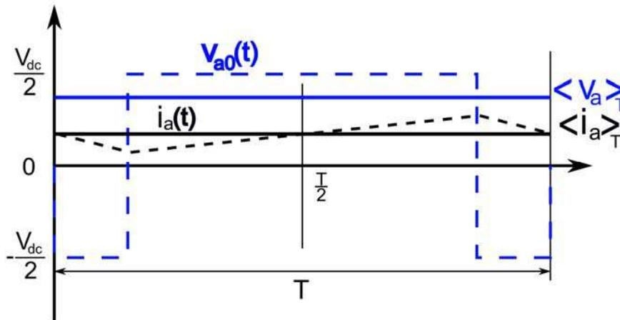
Figure II-44: Average current and harmonic current
