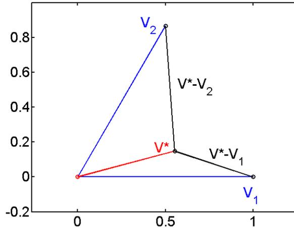
**Figure I-47: Harmonic voltage vectors**
