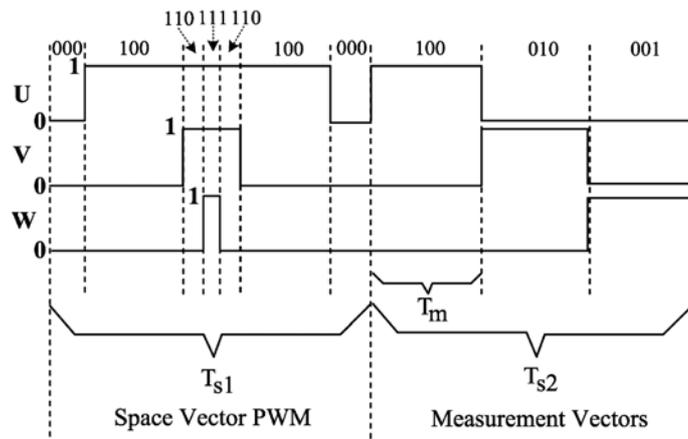
Figure II-41: Measurement vectors, [46]
