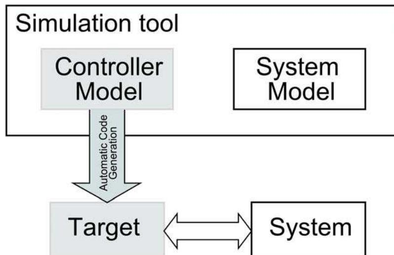
**Figure III-8: Rapid prototyping**
