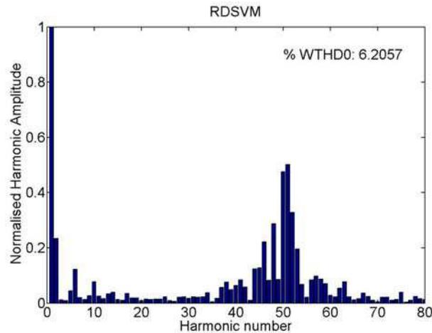
**Figure III-61: Vector controlled RSVM: Harmonic spectrum**
