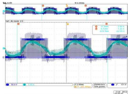
Figure III-48: Vector controlled DSVMMIN: Phase voltage and current
