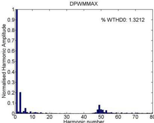
**Figure III-34: DPWMMAX: Harmonic spectrum**
