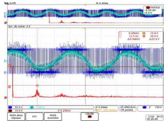
**Figure III-57: Vector controlled RSVM: Phase voltage and current**
