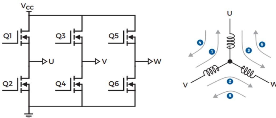
Figure 9. Three Half-Bridges with common node coils
