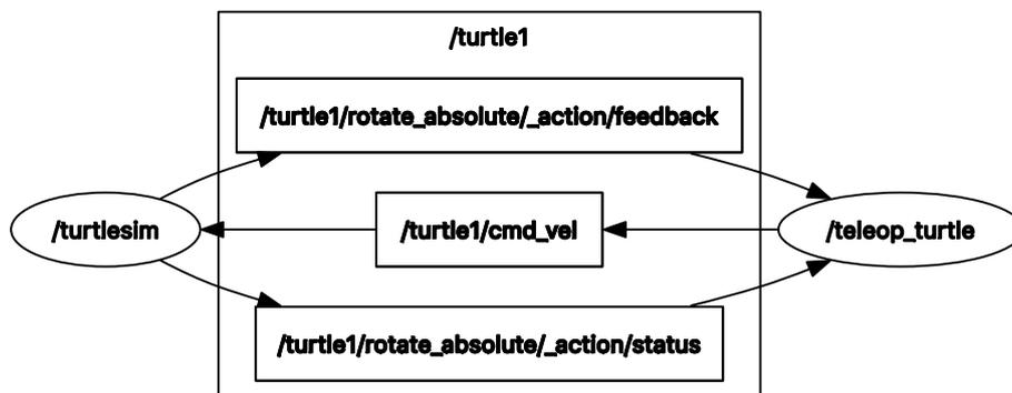
**Figure 2.1.** A simple ROS Computation Graph. Two nodes (represented as ellipses) (`/turtlesim` and `/teleop_turtle`) are running. The rectangles represent topics. The application is a part of the `turtlesim`<sup>1</sup> package.
