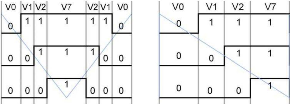
**Figure II-51: Triangle and sawtooth modulation**
