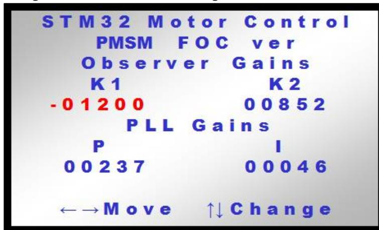
When the menu in *Figure 124: "LCD screen for setting the P term of the flux PID"* is displayed, the joystick can be moved to the right/left to navigate between the different gains. Pressing the joystick up/down will increment/decrement the gain highlighted in red color.
