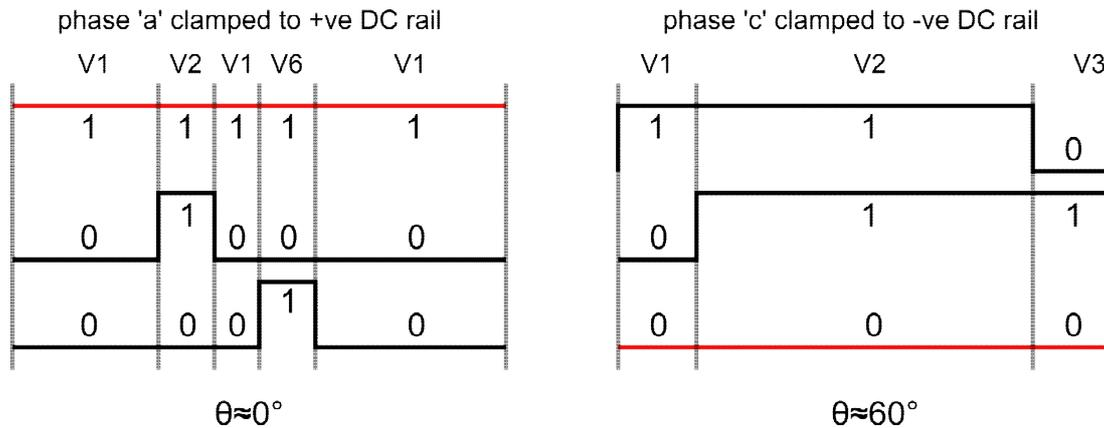
Figure II-53: Discontinuous PWM for phase current deduction
