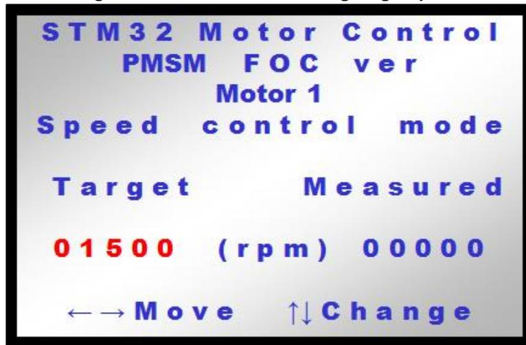
Like in the torque control mode, the motor is started/stopped by pressing the joystick or the KEY button.
