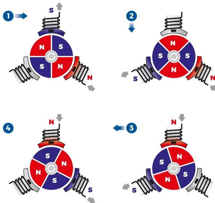
**Figure 4. Electronic commutation by energised windings**
