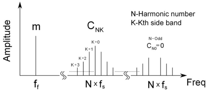
Figure I-40: Frequency Spectrum: PWM
