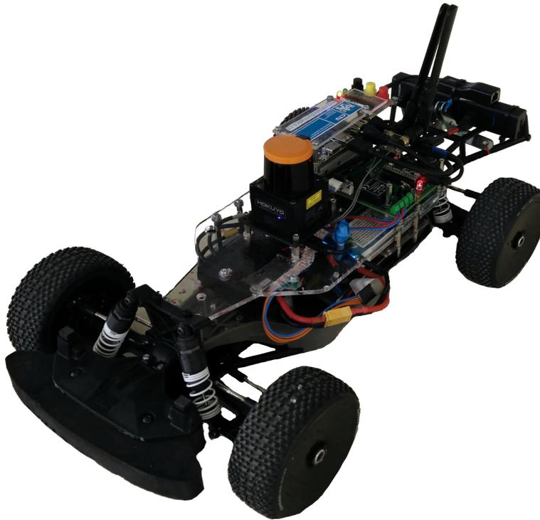
**Figure 4.2.** The CTU’s tx2-auto-3 F1/10 Model Car based on NVIDIA Jetson TX2.
