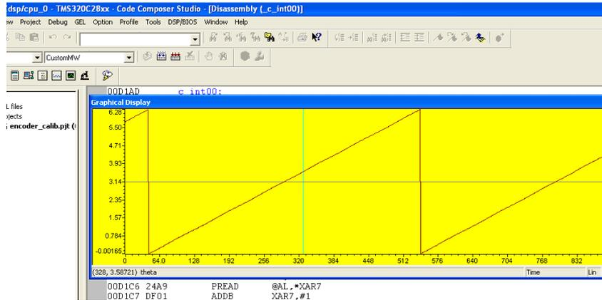
Figure III-18: Encoder verification
