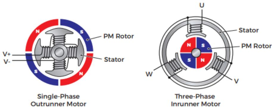
**Figure 3. Single-phase and three-motor**
