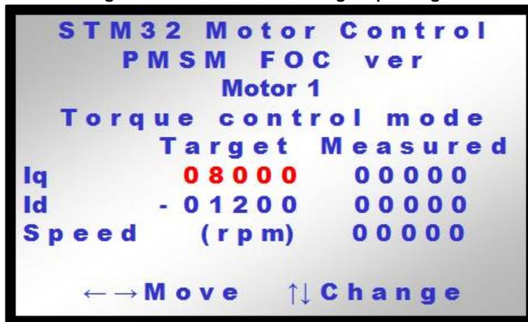
From the previous screen (*Figure 116: "LCD screen for Target Iq settings"*), if the joystick is moved to the right, the Target  $I_d$  current component becomes highlighted (in red). This parameter can now be modified by moving the joystick up/down. Once the motor Start command has been issued, the Target  $I_d$  can be changed in runtime while the measured  $I_d$  current component is shown in the Measured field.
