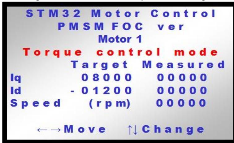
From the previous screen (*Figure 115: "LCD screen for Torque control settings"*), if the joystick is moved to the right, the Target  $I_q$  current component becomes highlighted (in red). This parameter can now be modified by moving the joystick up/down. Once the motor Start command has been issued, Target  $I_q$  can be changed in runtime while the measured  $I_q$  current component is shown in the **Measured** field.
