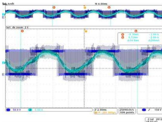
Figure III-47: Vector controlled DSVMMAX: Phase voltage and current
