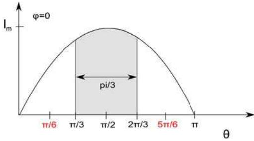
Figure II-7: Switching loss reduction  $\varphi=0^\circ$
