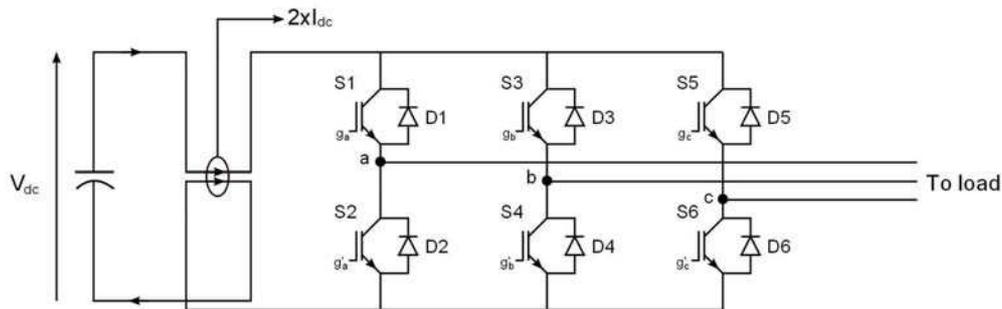
Figure II-46: Fault detection with one current sensor, [51]
