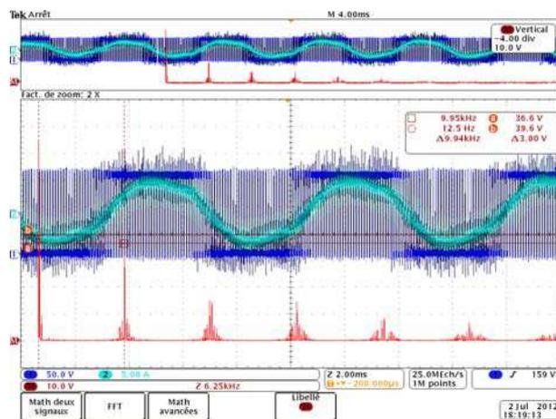
**Figure III-44: Vector controlled SVM: Phase voltage and current**
