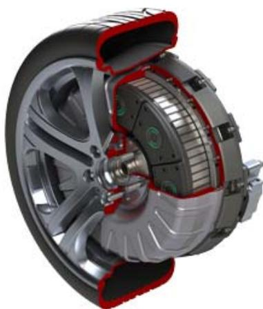
Figure 9: Protean in-wheel motor
