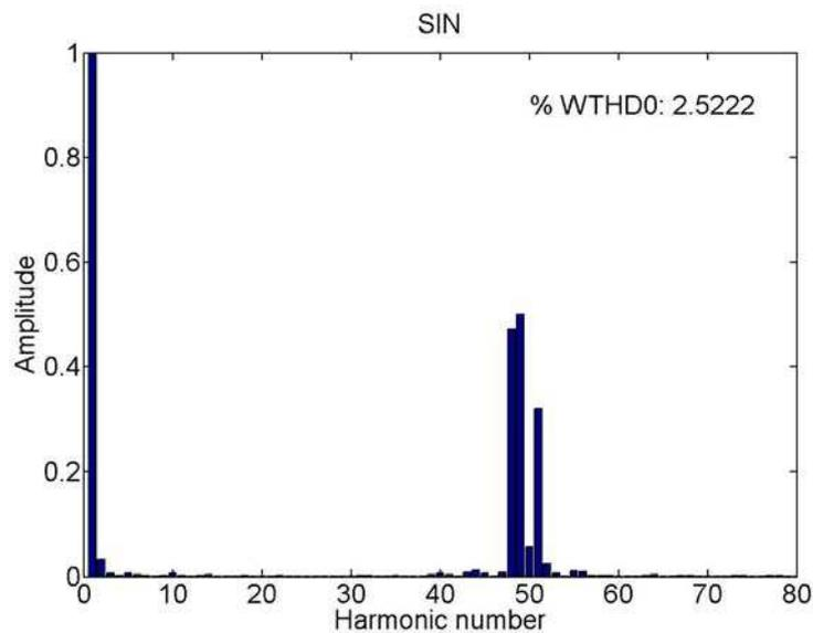
**Figure III-42: Vector controlled SPWM: Harmonic spectrum**
