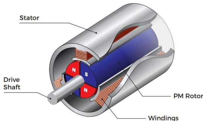
Figure 1. Axial view of a Brushless DC motor
