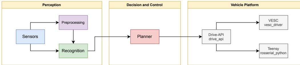
**Figure 4.7.** a high-level overview of a typical data flow is depicted in the the CTU F1/10 platform.
