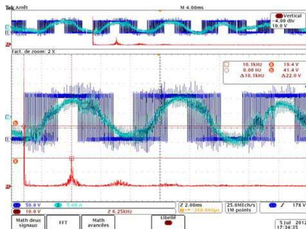
**Figure III-60: Vector controlled RDSVM: Phase voltage and current**
