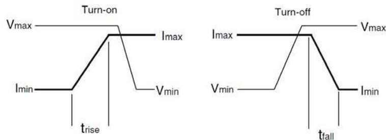
Figure I-32: Hard Switching
