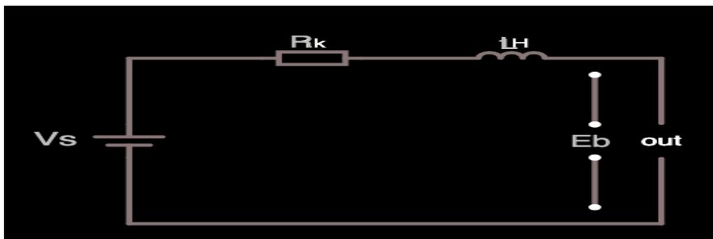
Figure 2: DC motor circuit.  $V_s$  is the voltage in.  $R_k$  is the motor resistance,  $L_h$  is the inductance,  $E_b$  is the back EMF voltage.
