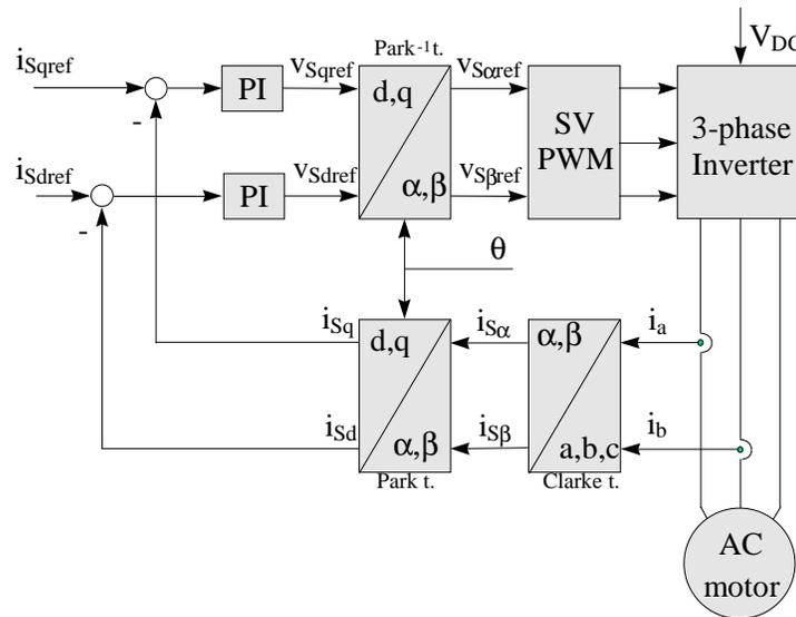
**Figure 4: Basic scheme of FOC for AC-motor**
