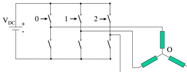
**Figure 8: Basic scheme of 3-phase inverter and AC-motor**
