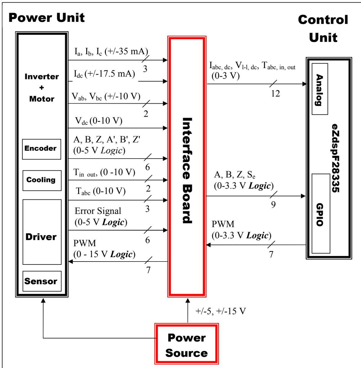
Figure III-11: Schematic diagram of the interface circuit
