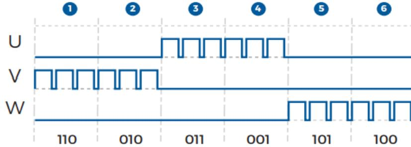
**Figure 10. PWM input applied to each phase**
