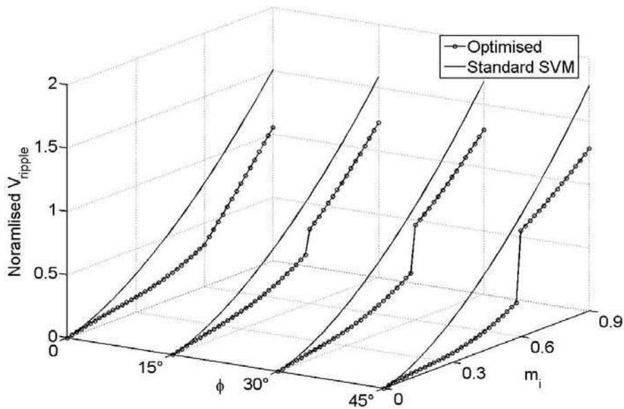
Figure II-61: RMS input voltage ripple
