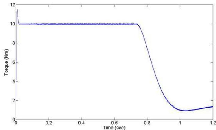
**Figure II-17: EDSVM torque response**
