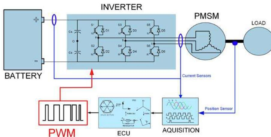
Figure I-1: Schematic diagram of an Electric Drive
