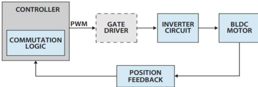
**FIGURE 11. Basic control diagram of a brushless DC motor**
