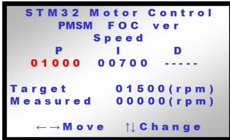
Like for the previous menus, either of the P or I coefficients can be selected (highlighted in red) by moving the joystick to the right/left. The desired values can then be changed (incremented or decremented) by pressing the joystick up/down.
