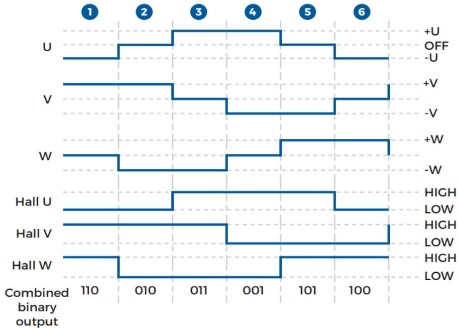
**Figure 5. Phase excitation and Hall-sensor outputs**
