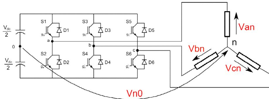
**Figure I-6: Inverter fed floating neutral 3-Phase load**
