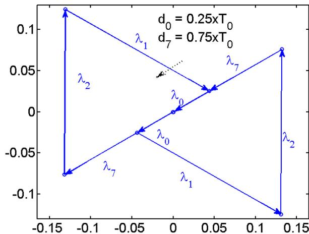
**Figure II-26: Harmonic flux,  $\lambda_h$  for  $d_0 \neq d_7$**
