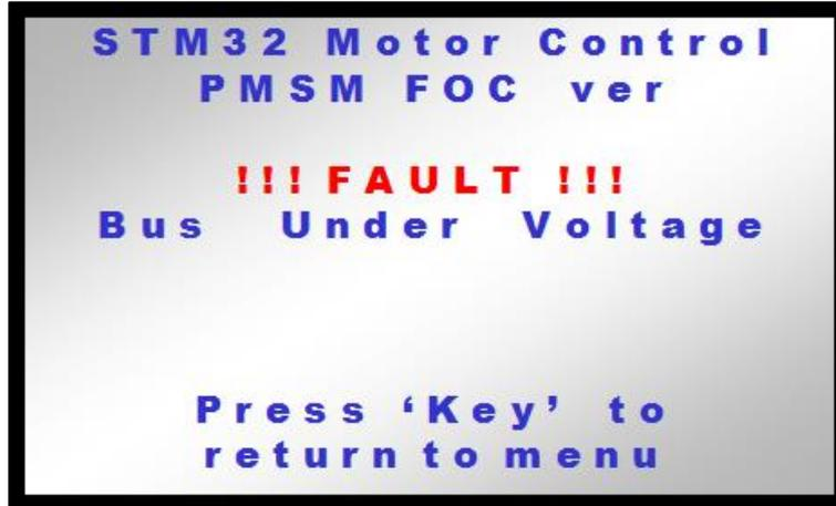
The message "Press 'Key' to return to menu" is visible only if the source of the fault has disappeared. In this case, pressing the 'Key' button causes the main state machine to switch from the Fault occurred state to the Idle state.
