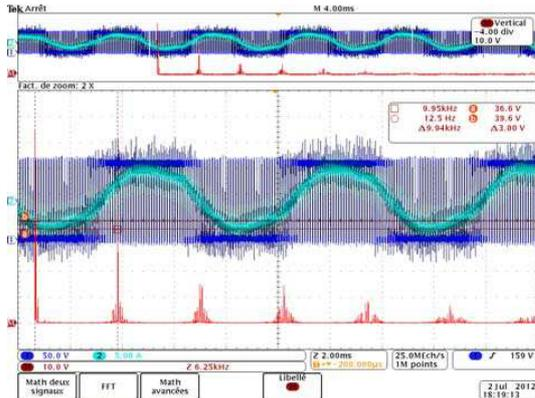
**Figure III-56: Vector controlled SVM: Phase voltage and current**
