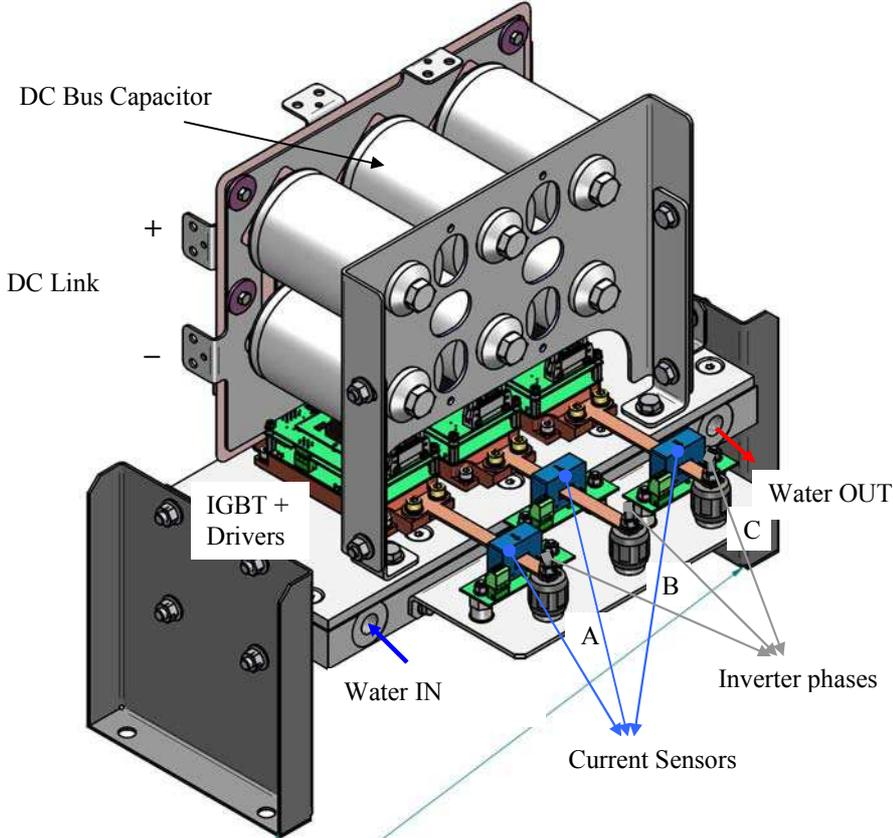
**Figure III-3: Inverter module**
