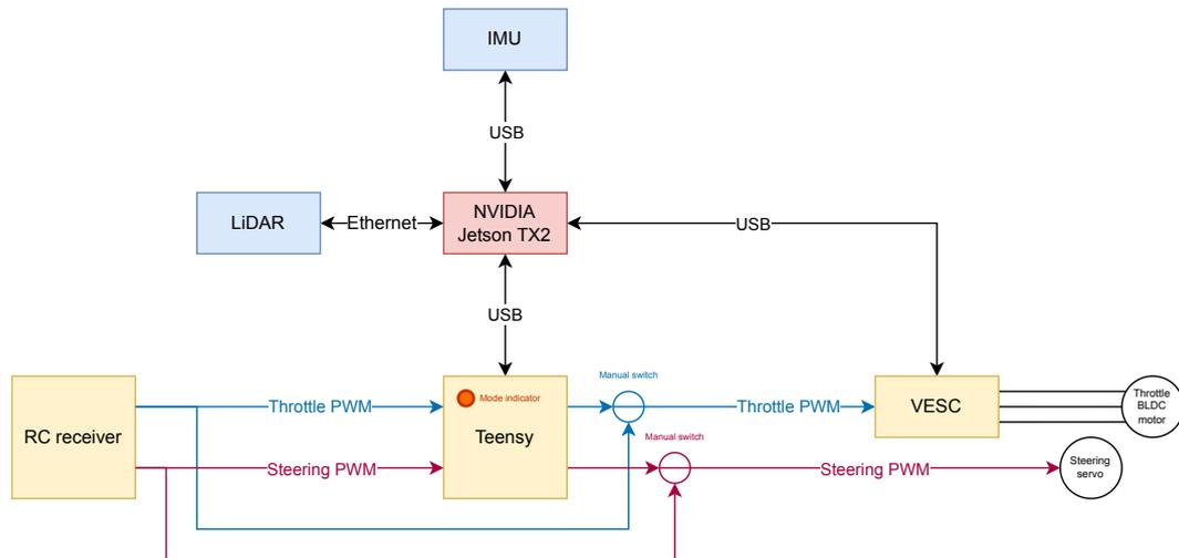
**Figure 4.3.** Overview of main components with depicted methods of communication. The yellow blocks are part of the low-level system, which always works independently of the main high-level system (NVIDIA Jetson TX2).
