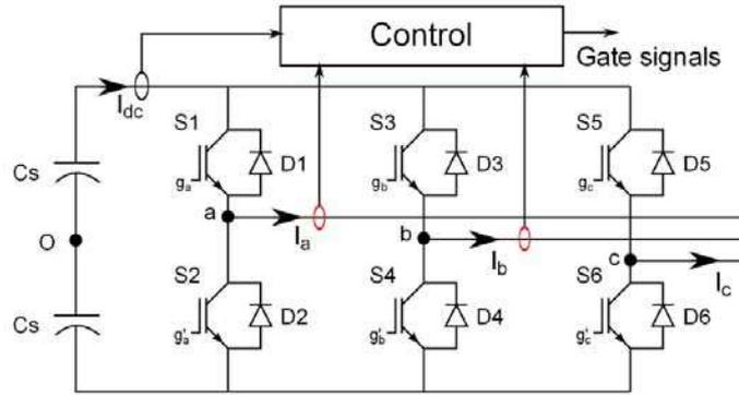
**Figure II-38: Three phase Inverter and current sensors**
