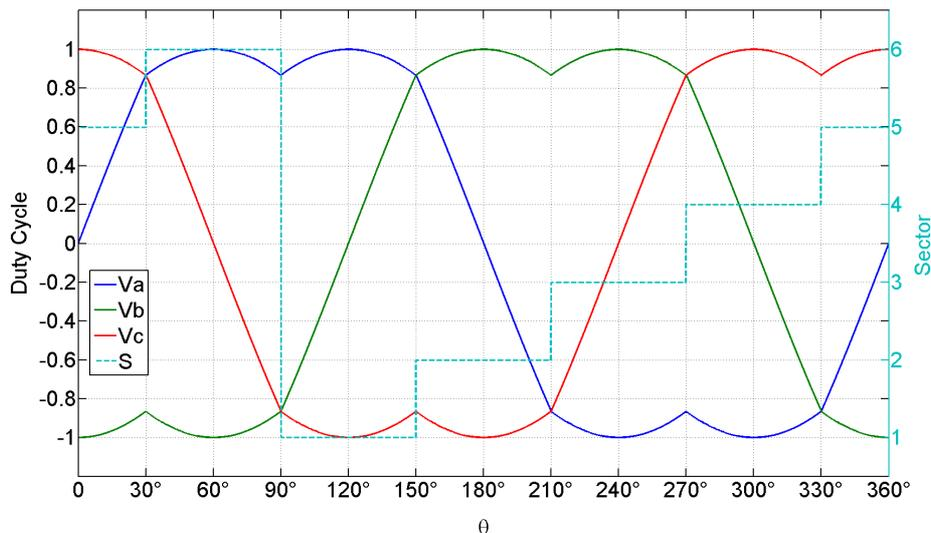
**Figure I-17: SVM; modulation function and corresponding sectors**
