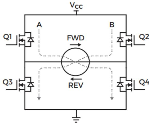
Figure 8. H-bridge inverter circuit
