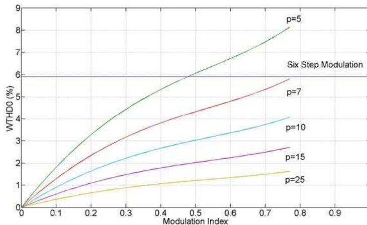
Figure III-20: WTHD0 for SPWM for different pulse ratios
