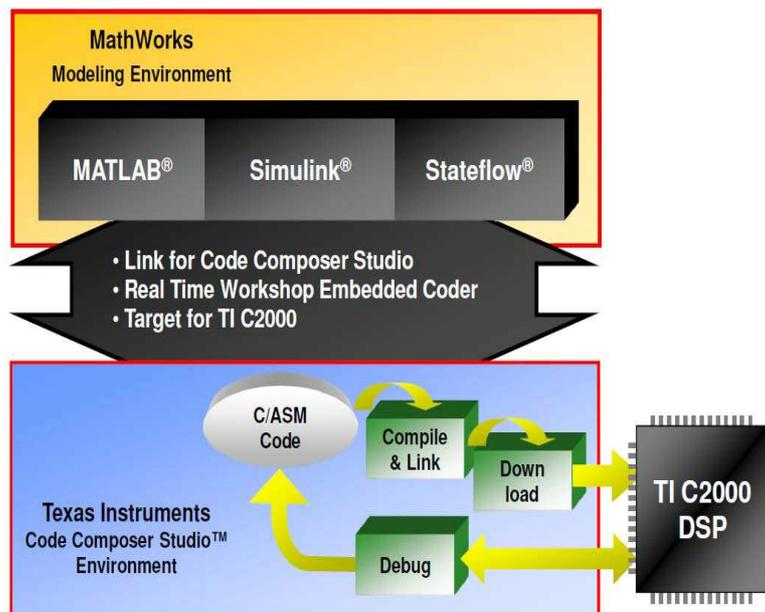
**Figure III-10: Automatic code generation**
