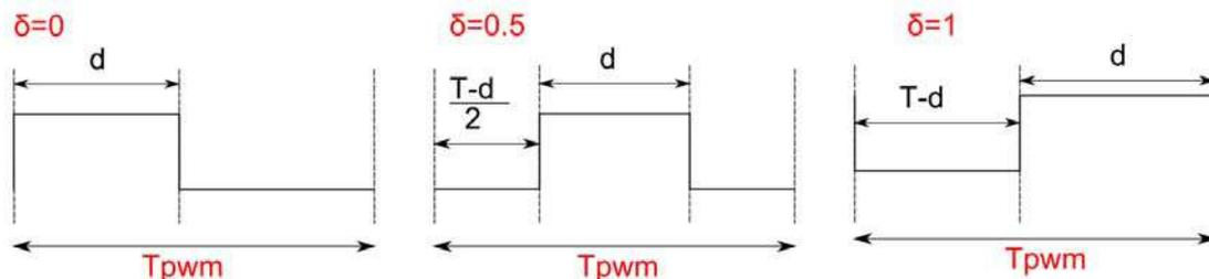
**Figure I-27: Pulse positioning**
