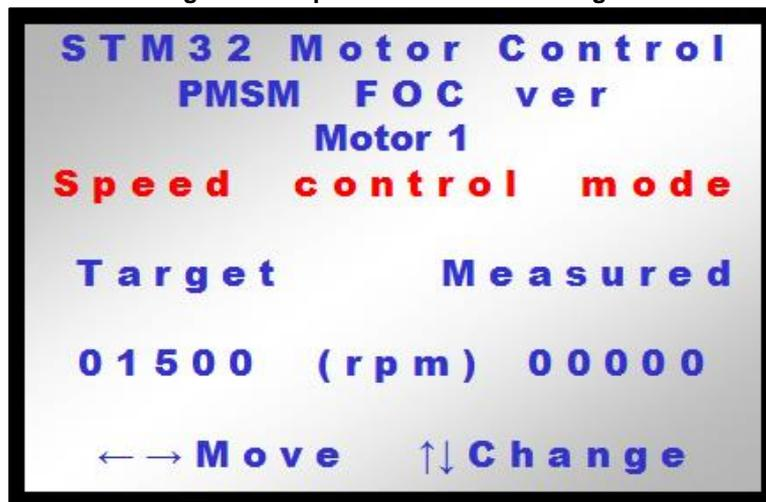
From the menu screen shown in Figure 118: "Speed control main settings", moving the joystick to the right selects the Target speed (parameter highlighted in red). Once selected, the parameter can be incremented/decremented by moving the joystick up/down. The motor can then be started simply by pressing the joystick. When the motor is on, the target speed can still be modified.
