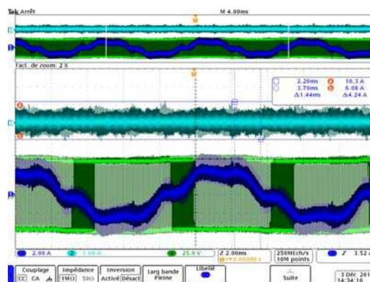
Figure I-34: Leakage current (top),  $I_a$  and  $V_{a0}$
